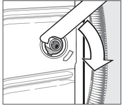
■ Turn the right shipping strut counterclockwise 90° with the enclosed combination wrench.
